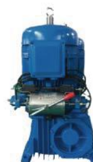
Escalator drive main engine
